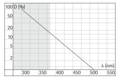
Relative damage factor D of optical radiation as a function of wavelength  $\lambda$ . Damage decreases exponentially through the wavelengths including the majority of the range of visible radiation.
